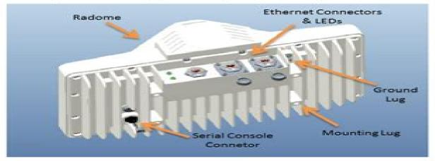
The side where the mounting lugs and serial port are located is referred to as the "back", since it is the side that will be against a wall or mast when IBR is mounted.
