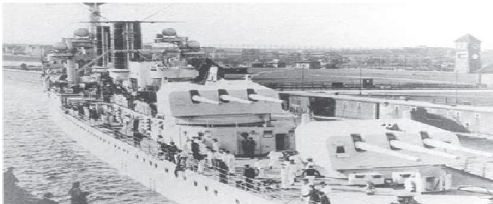
Karlruhe in a Wilhelmshaven lock after commissioning. Notice the dark-painted funnels. The photograph gives a good view of the unorthodox alignment of 'B' and 'C' turrets off the centerline. In accordance with German naval tradition, 'C' turret bore the name SMS Goeben .
