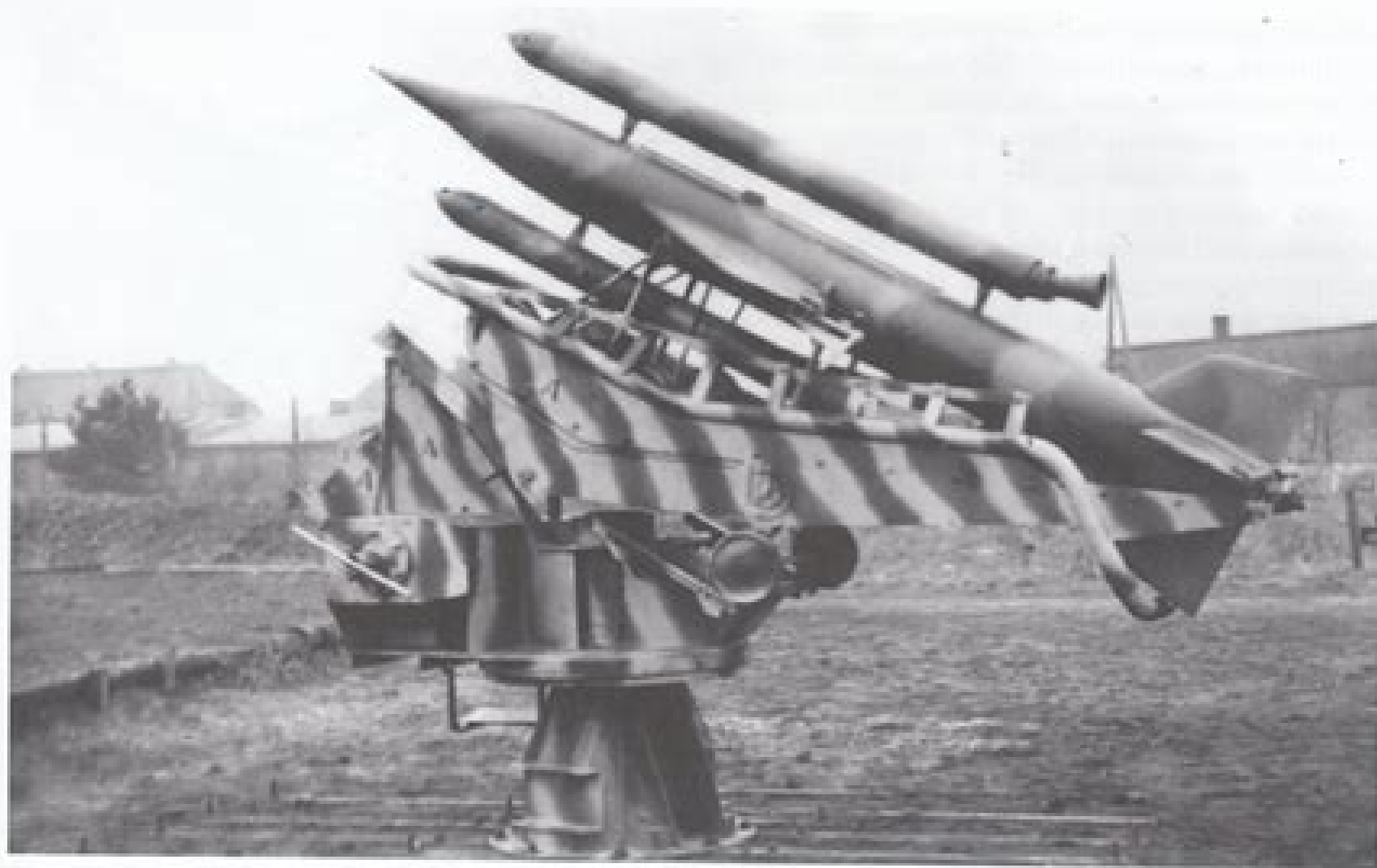
The Henschel Hs 117 V-1 Schmetterling used a traversable launcher during the test phase.
