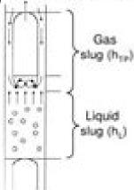
$$h_{TP} = F_p h_L \left[ 1 + 0.55 \left( \frac{x}{1-x} \right)^{0.1} \left( \frac{1-F_p}{F_p} \right)^{0.4} \left( \frac{Pr_G}{Pr_L} \right)^{0.25} \left( \frac{\mu_L}{\mu_G} \right)^{0.25} \left( I^* \right)^{0.25} \right]$$
