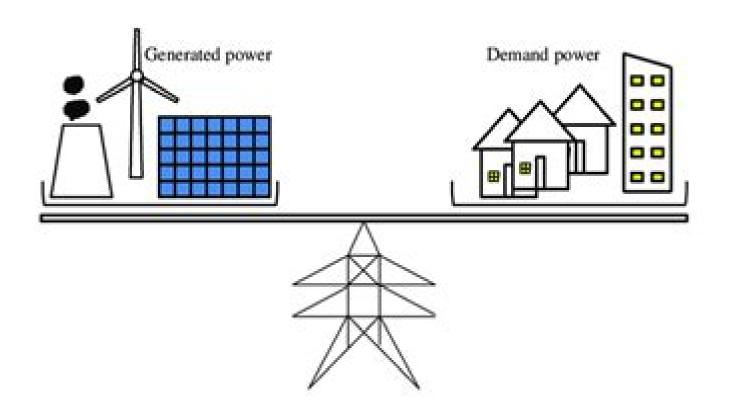
re 1. Power Load Balance. The balancing between the generated and consumed power, this is main tasks of the distribution power system for producing power with good quality.
