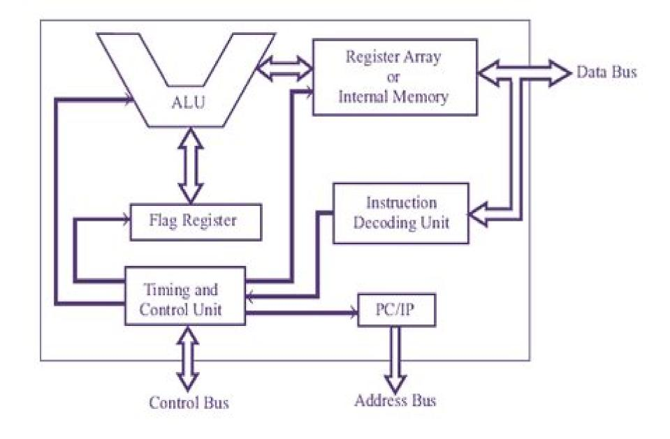
Fig: Block Diagram of Basic Functional Blocks of a Microprocessor
