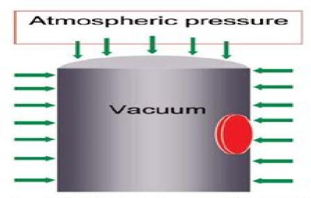
Storage tanks and railcars are particularly susceptible to damage, but it can also happen to process vessels that are only rated for low pressures or very large pipes.
